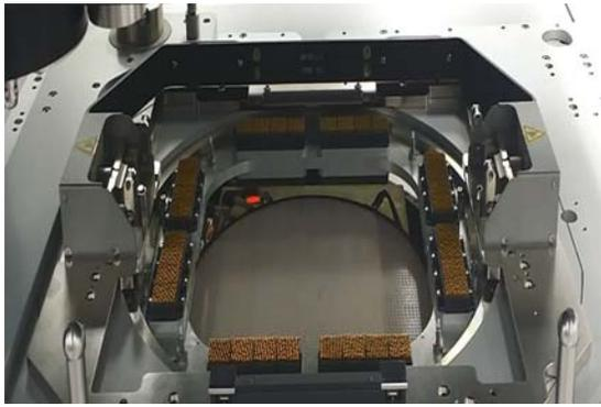
**Figure 7.** Indexing of eWLCSP™ carrier in wafer test of FlexLine™
