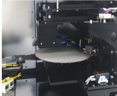
**Figure 6.** Pre-aligner station where the wafer notch is detected and wafer ID is read of eWLCSP carrier in prober system in FlexLine
