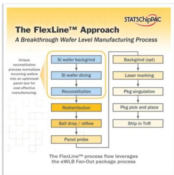
Figure 1. The FlexLine Process Flow
