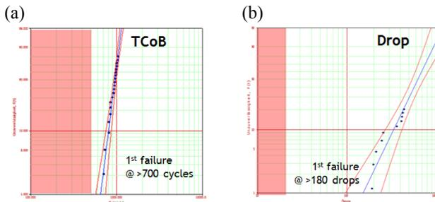
**Figure 3.** Weibull plots of board level reliability of WLCSP+ : (a) TCoB and (b) drop test
