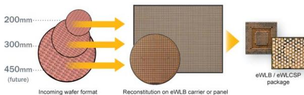
Figure 2: The FlexLine approach can process multiple silicon wafer diameters on the same manufacturing line to produce both fan-in and fan-out packages.
