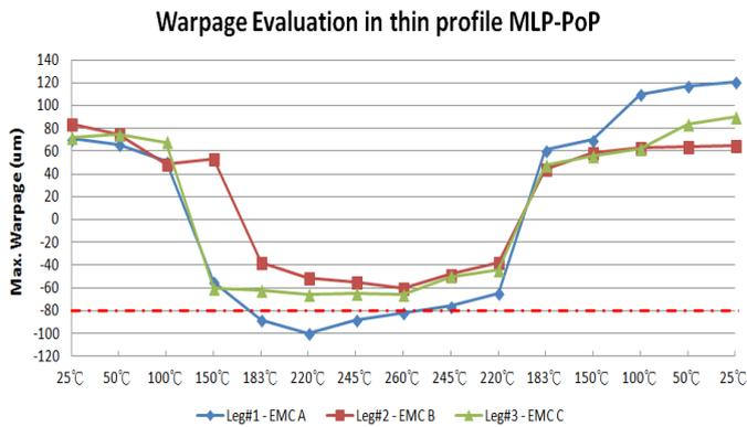
Fig. 7. Max. warpage behaviors in OM MLP-PoP with 1/2/1 substrate (S/S: 10ea in each leg)
