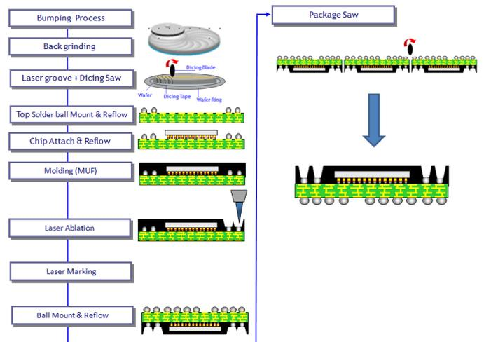
Fig. 6. Process flow of MLP-PoP bottom package with MUF
