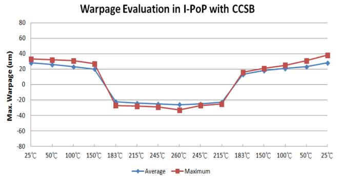
Fig. 14. Average and maximum warpage behaviors in I-PoP with CCSB interconnections (S/S: 10ea in each leg)
