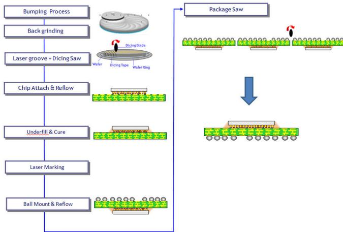
Fig. 4. Process flow of BD-PoP bottom package
