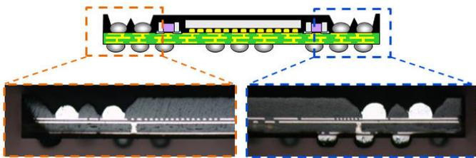
Fig. 8. Cross-sectional view in thin profile OM MLP-PoP
