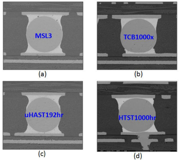
Fig. 13. Package level reliability result in I-PoP with CCSB interconnections.
