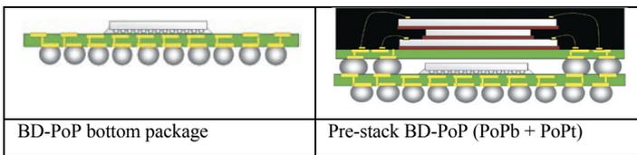
Fig. 1. Schematic of bare die package-on-package (BD-PoP)
