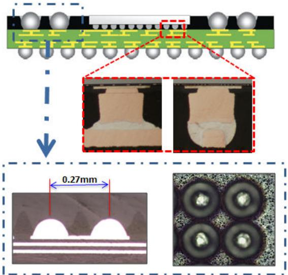
Fig. 9. Cross-sectional view for 0.27mm top ball pitch in ED MLP-PoP
