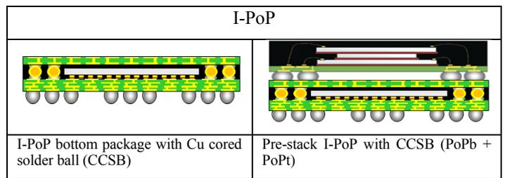
Fig. 3. Schematic of interposer package-on-package with Cu cored solder ball (I-PoP with CCSB)
