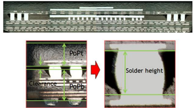
Fig. 10. Pre-stack result in ED MP-PoP with 0.27mm top ball pitch
