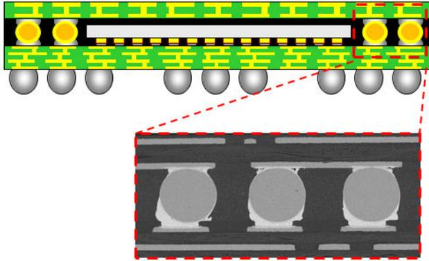
Fig. 12. Cross-sectional view for I-PoP with Cu cored solder ball (CCSB) interconnections.
