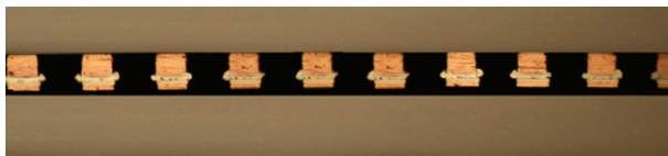
fcBGA with thermal compression bonded microbumps on the TSVs
