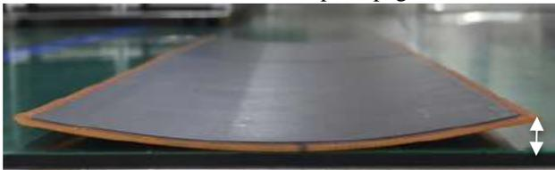
Figure 12: Typical strip warpage shape from TV 2 DOE
