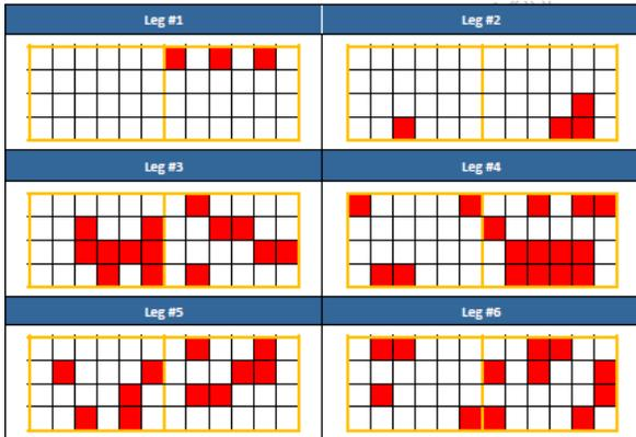
Figure 12: Mold bleed on pad unit mapping of the mold bleed units from the TV 2 evaluation matrix
