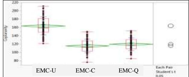
Figure 14: Coplanarity data by EMC type
