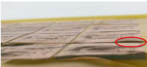
Figure 8: Gap between substrate and tape observed after the lamination process from the TV1-1 evaluation
