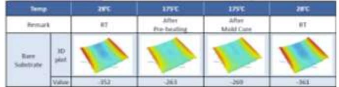
Figure 10: Ultra thin substrate thermal moiré warpage plots for room-pre-heat-room temperature transitions
