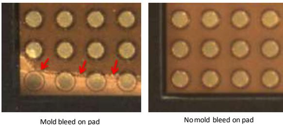
Figure 9: Examples of mold bleed in the substrate pad
