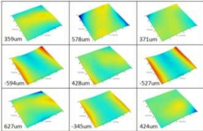
Figure 2: 17X17mm body size ultra thin bare substrate warpage data at 25<sup>0</sup>C
