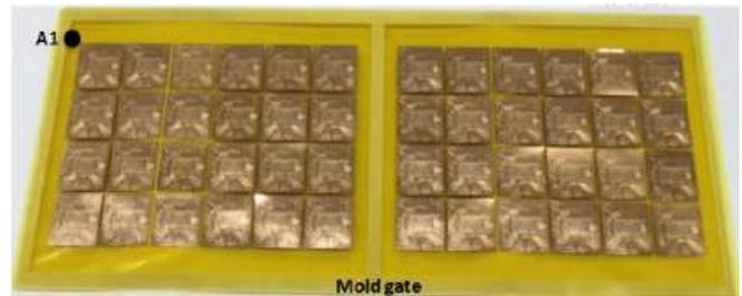
Figure 6: Singulated ultra thin substrates placed on the polyimide tape fixed to a window carrier prior to the reconstitution process.
