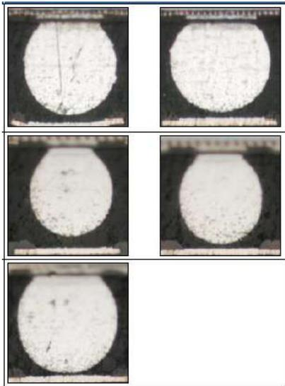
Figure 16: TV 2 non-wets due to excessive substrate warpage. Some of the functionally good parts were also cross-sectioned and checked for bump integrity and other anomalies in the package. No bump crack or tearing and EMC crack or separation was observed in the picture shown in Figure 17.
