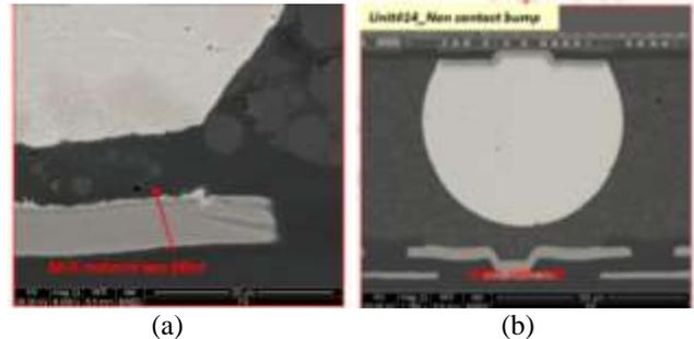
Figure 11: (a) A brittle separation at the bump-to-bump pad interface with the MUF material filled in and (b) a non-wet
