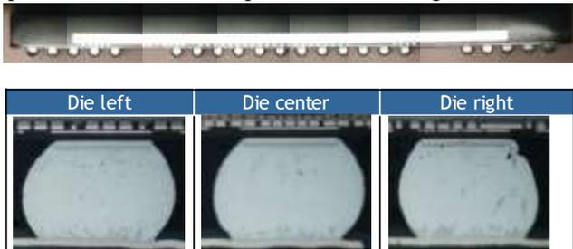
Figure 17: No bump crack or non-wet observed with good units from TV2 DOE
