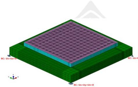
Figure 3. FEA Model of eWLB Package
