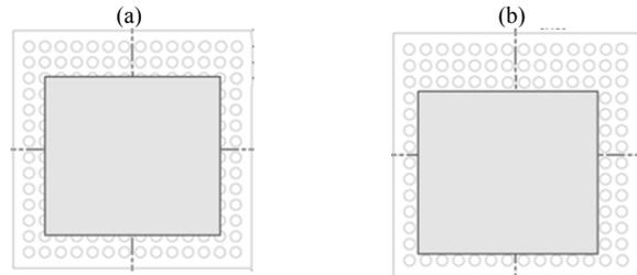
Figure 7. Die position in eWLB (a) Centred and (b) Off-centred
