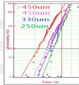
Figure 6. Weibull Plot of Daisychain TV of TCoB Reliability Tests.
