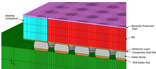
Figure 4. Internal Cutout View of eWLB Package
