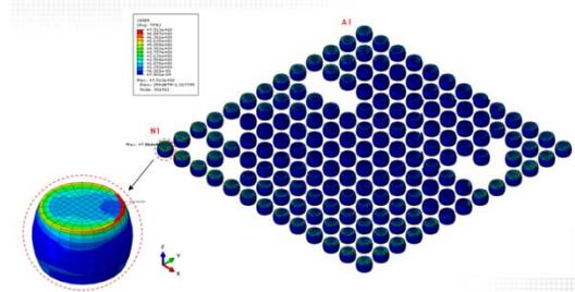
Figure 5. Creep Strain Distribution Plot for Solder Joints of 475um Thick eWLB at End of Third Cycle
