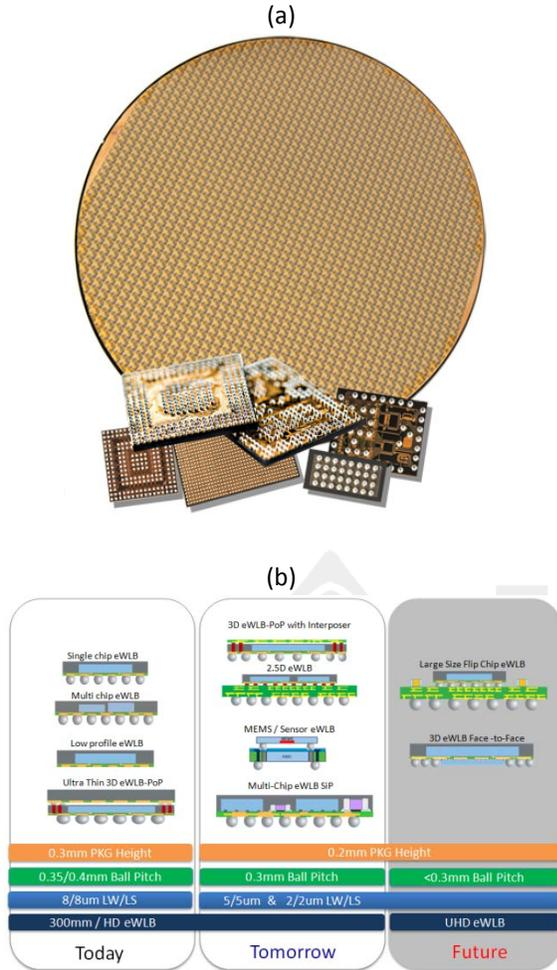
Figure 1. (a) 300mm eWLB carrier and eWLB packages, and (b) evolution of eWLB technology from 2D to 2.5D/3D packaging solution
