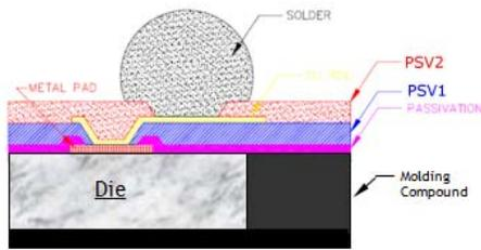
Figure 2 . Cross-section Diagram of eWLB with 1L-RDL
