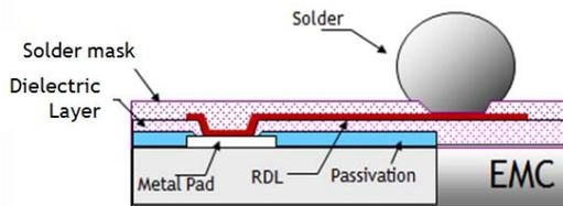
Figure 3. Schematics of eWLB package.
