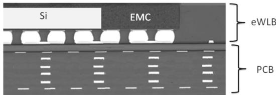
Figure 5. Schematics of cross-section of eWLB mounted PCB of Fig. 6.
