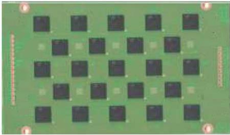
Figure 4. Board level reliability test board with surface mounted eWLB packages.
