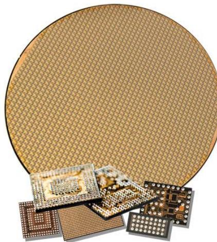
Figure 1. 300mm eWLB carrier and various units.
