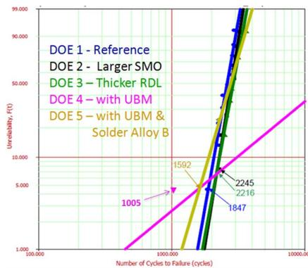
Figure 6. Weibull plot of TCoB DOE study with NSMD PCB. Each no. indicates the first failure cycle in each DOE.
