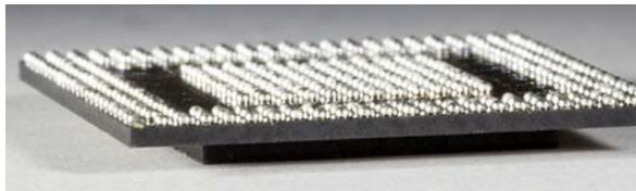
**Figure 10.** Top: concept illustration of double-side eWLB. Middle: SEM picture of a double-side eWLB with PCB-bars. Bottom: a double-side eWLB with a smaller package stacked onto it (upside down).
