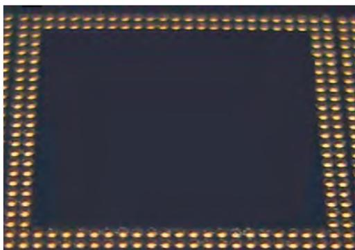
Figure 5. Micrograph of top view of eWLB-PoP, after laser ablation process to form via hole in eWLB.
