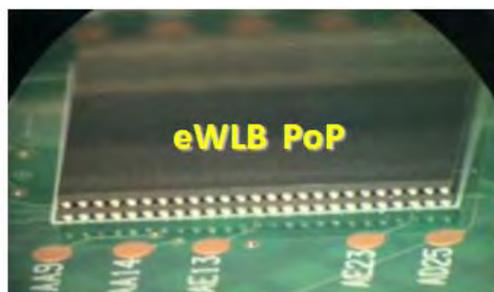
Figure 7. Board level reliability test samples of eWLB-PoP mounted on PCB
