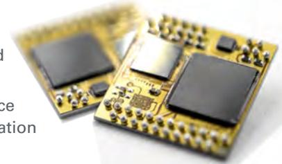
With these advantages, SiP is able to address some of the limitations of silicon (Si) level integration (commonly known as System-on-Chip or SoC), including design complexities, long development cycles, manufacturability, intellectual property (IP) and legal issues, longer time-to-market and higher costs. SiP provides a high performance packaging solution that is scalable, cost effective and can be easily implemented in an electronic device.
